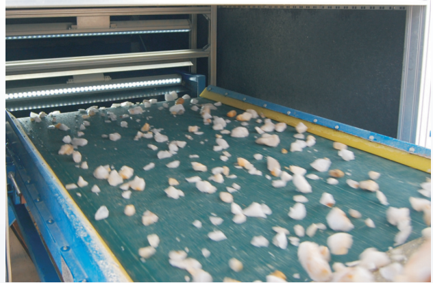
Inlet to the OSX-1000 separator
